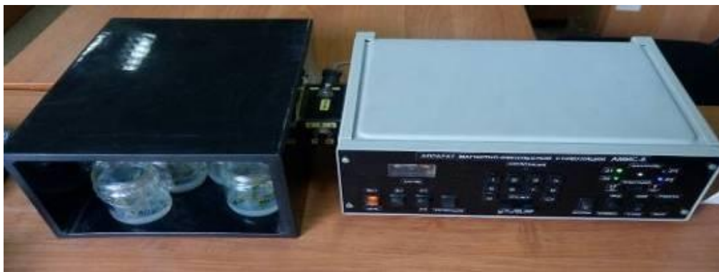
Figure 1. Magnetic pulse processing of apple clonal rootstock 62-396 explants using the AMIS-8 apparatus.
