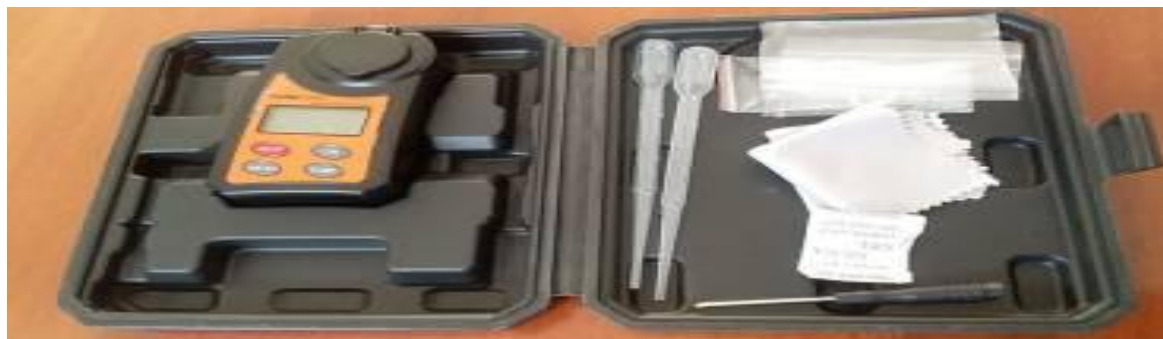
Figure 2. Ruoshui 2GHS refractometer (Sánchez-Pérez et al. , 2008).
