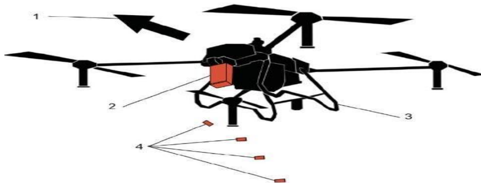
Figure 2. Capsule release mechanism using the unmanned aerial vehicle (UAV)-based system: 1) movement direction of the UAV, 2) spreader device, 3) UAV, and 4) capsules with entomophage eggs.
