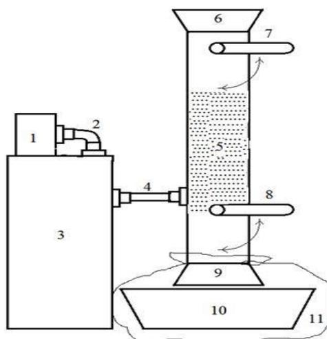
**Figure 1.** Semi-industrial ion-cavitation process line. 1: compressor, 2: air piping, 3: ion-ozone unit, 4: piping of ion-ozone mixture, 5: cavitation unit, 6: grain filling pipe, 7: grain filling valve, 8: pressure relief valve, 9: grain discharge pipe, 10: tank - grain collector, 11: grain trap.
