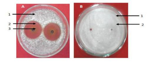
**Figure 2.** Inhibition zone formed around the well diffusion filled with partitioned leaf extract of *Ficus septica* of methanol phase (A) and hexane phase (B). (1 = mycelium of C. acutatum, 2 = well diffusion, and 3 = inhibition zone).
